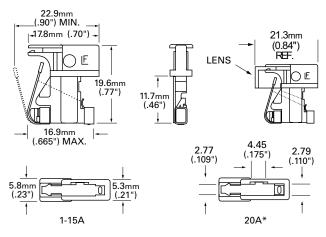
\*20A Fuseholder must be used. Fuse is keyed to prevent insertion in lower rated holders. 20A Fuseholder is designed to accept all ratings up to 20 amperes.
