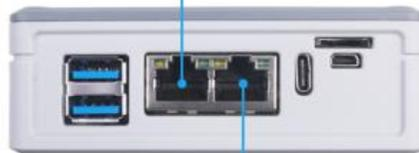
Microchip LAN7800 (USB 3.0 to Gigabit Ethernet Bridge) - USB3.0 extended from PCIe of CM4
