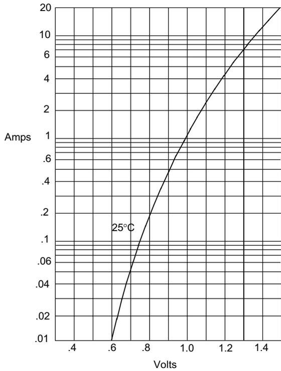
Instantaneous Forward Current - Amperes *versus*
