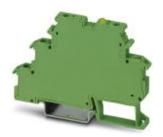
Input solid-state relay, with DC voltage output push-pull, transmission frequency: 100 kHz, with light indicator and protective circuit in input and output circuits, input: 24 V DC, output: 14 - 30 V DC/50 mA
