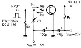
$10I_{B1} = -10I_{B2} = I_0 = 500 \text{mA}$ (For PNP, the polarity is reversed.)
