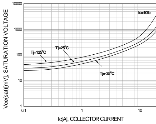
Figure 4. Collector-Emitter Saturation Voltage
