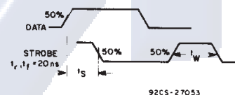
Fig. 15 - Data setup time and strobe pulse duration.
