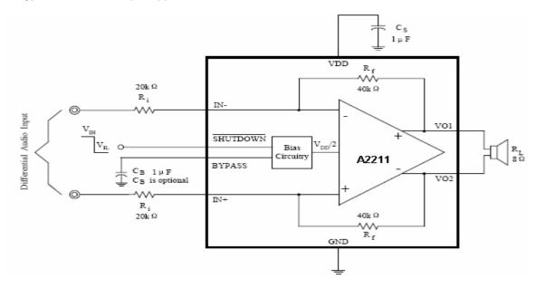
2. Differential Input application with Input Capacitors
