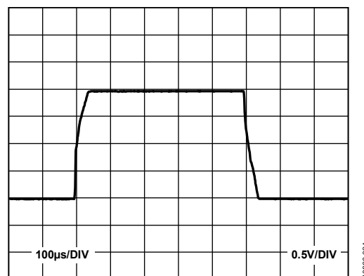
Figure 24. Operational Amplifier Large Signal Transient Response
