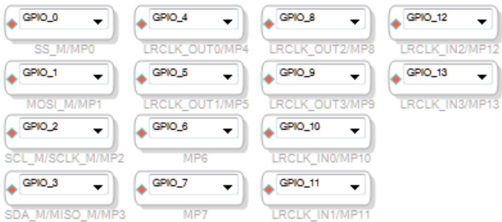
Figure 77. Complete Set of General-Purpose Outputs in SigmaStudio
