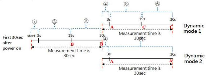
After sensors are in dynamic working mode, start measuring every 30s. The sensor starts the measurement for the first 3 seconds.
