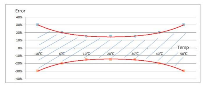
Measured error: under  $25^{\circ}C \pm 2^{\circ}C$ ,  $50\pm 10\%$  RH,  $0\sim 1000 \mu g/m^3$ , consistency and accuracy of PM2.5 is  $\pm 15\%$  reading or  $\pm 15 \mu g/m^3$ , whichever is larger.
