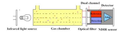
The infrared light source radiates infrared light which passes through the measured gas in the optical path and narrow band filters, then reaches the infrared detector. By measuring the intensity of the infrared light arriving at the infrared detector, the concentration of the measured gas can be calculated.
