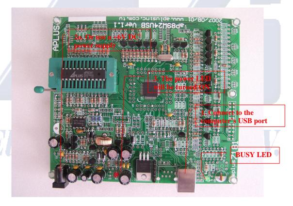
If the computer's USB ports are already connected to many USB devices, it will happen that the USB port does not have enough current output to drive the aP89W20 programmer. In this situation, an external DC +6V power supply should be used instead of the USB.
