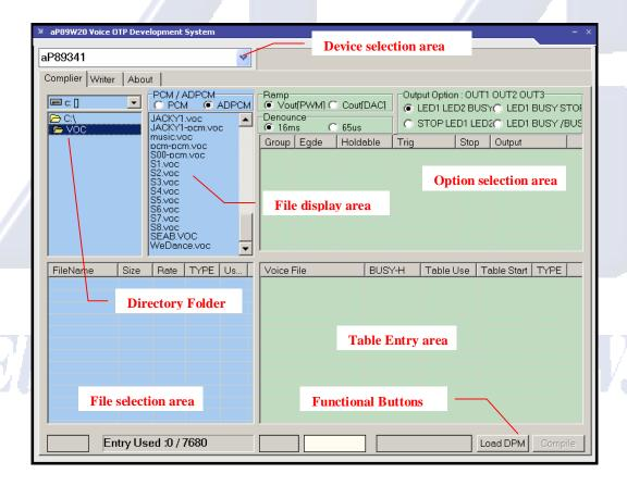
Voice data and user selectable options must be set up and combined together to form a DPM file before it can be programmed into the Voice OTP device. The following procedures describe step by step how to compile the voice data and options to produce the DPM file for programmed into the chip.
