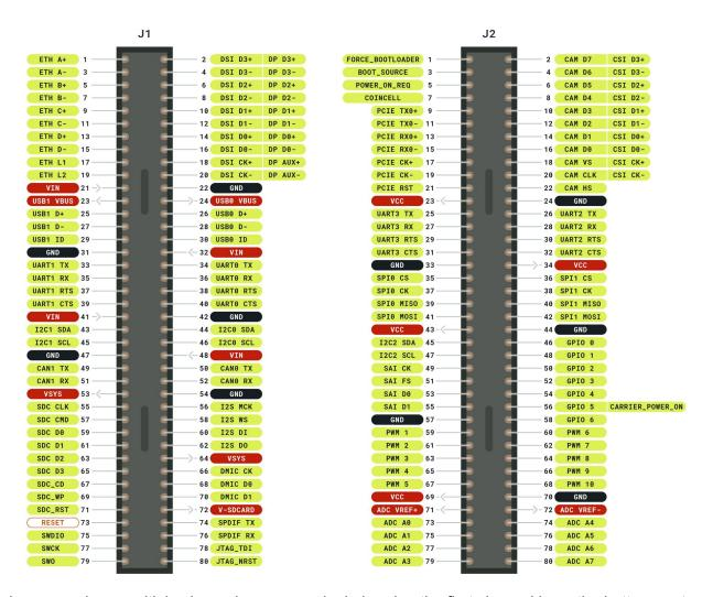
In cases where multiple channels are on a single header, the first channel is on the bottom part of the header and the section channel is on the top part of the header. The order of the channel is determined by the silkscreen markings.
