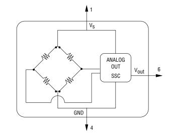
Note: Power supply decoupling and output filtering included.
