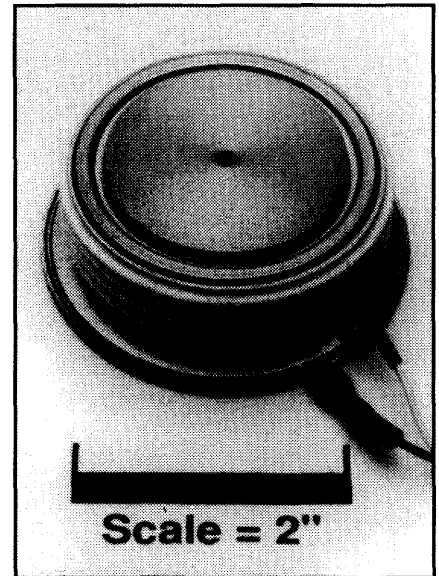
C451 Phase Control SCR 1500 Amperes Average, 2400 Volts
