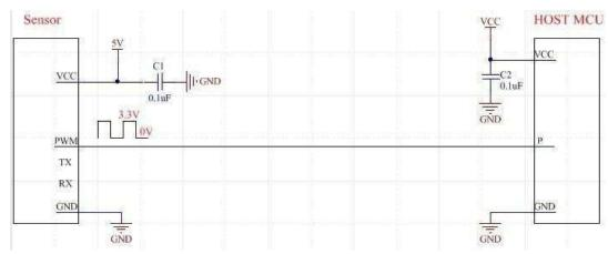
Case2. 5V level and 3.3V level conversion circuit
