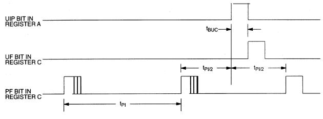
$t_{Pl}$  = PERIODIC INTERRUPT TIME INTERNAL PER TABLE 1  $t_{BlJC}$  = DELAY TIME BEFORE UPDATE CYCLE = 244  $\mu s$
