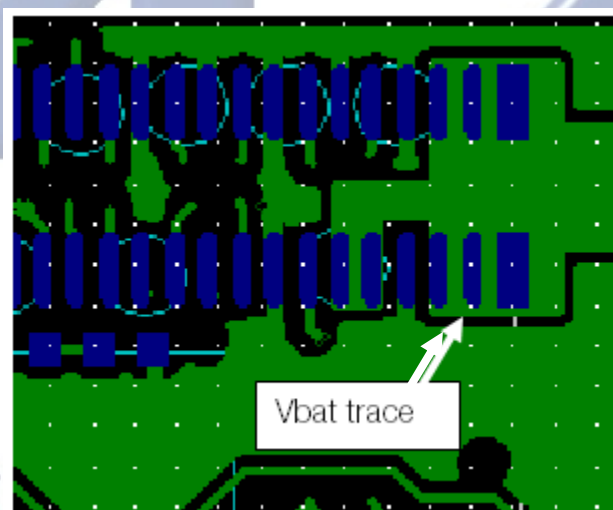
Figure 7 - Example of GOOD Vbat layout
