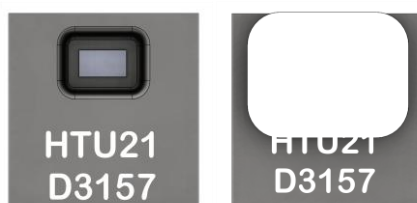
Laser marking on HTU21D(F) sensor
