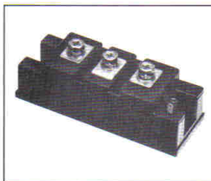
KR224575 Chopper Darlington Transistor Module 75 Amperes/600 Volts
