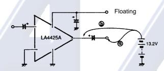
The power pin is in a floating state when a power capacitor is connected, so if  $+V_{CC}$  touches output lines ⓐ and ⓑ, the upper power transistor inside the IC will be damaged.
