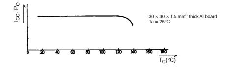
T.S.D is capable of starting operation at Tc 120 to 130°C. When this is converted to junction temperature (Tj) according to the formula below.
