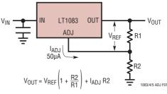
Figure 1. Basic Adjustable Regulator
