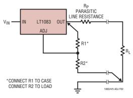
Figure 2. Connections for Best Load Regulation
