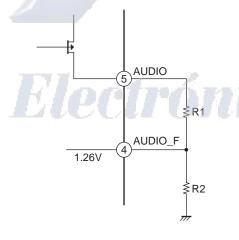
The AUDIO\_F voltage is determined by the internal band gap voltage of the IC (typ = 1.26V).
