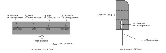
• Frame diagram (LV5680P) \*In the system power supply other than LV5680P, pin assignment may differ.
