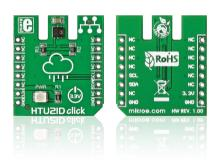
HTU21D click<sup>™</sup> carries a high-precision, easy-to-use relative humidity sensor with temperature output. The sensor is plug and play, requiring no calibration to use. The measurement range of HTU21D click<sup>™</sup> is from 0 to 100 percents of relative humidity, and -40 to +125 degrees of Celsius. The board communicates with the target microcontroller through mikroBUS™ I2C lines: SCL and SDA (data). It uses a 3.3V power supply only.
