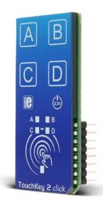
**TouchKey 2 click** has four capacitive pads powered by ATtiny817 which has an integrated touch QTouch® controller. The click is designed to run on a 3.3V power supply. The four LEDs onboard the click indicate when the Key (Pad) is pressed. TouchKey 2 click communicates with the target microcontroller over UART interface (SPI interface is optional).
