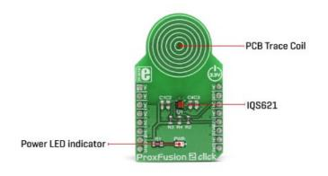
The IQS621 IC does not sacrifice any feature in favor of having multiple sensors on the same chip; on the contrary, it offers all the key features commonly found on other stand-alone sensors. The sensitivity of IQS621 is improved by using a regulated and stable internal power supply, along with the Automatic Tuning Implementation (ATI) technology, which provides consistent readings, regardless of environmental conditions.
