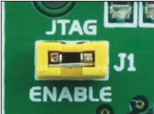
Figure 3-5: JTAG is enabled
