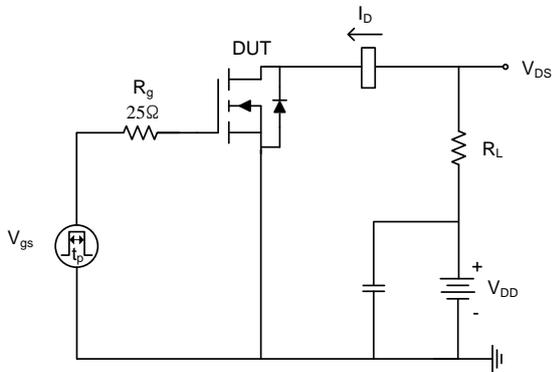
Fig17-1. Switching time test circuit for resistive load
