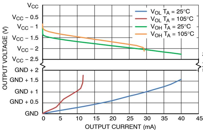
Figure 9. Output Voltage Swing vs. Output Current
