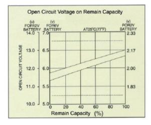
The above graph shows the remain capacity of NP and GM Series batteries by measuring the open circuit voltage.
