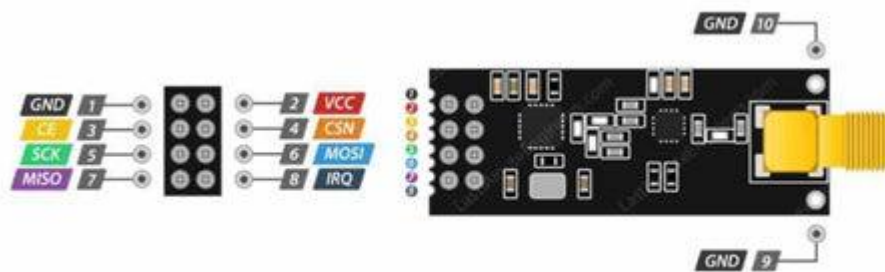
nRF24L01+ PA/LNA Pinout
