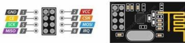
nRF24L01+ Pinout
