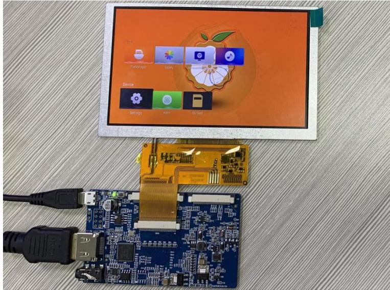
4) When the Android system is started for the first time, it is normal for the screen display to be jittery or blurry, because the default HDMI resolution of the Android system is 1080p, but the TFT LCD screen does not support this resolution. After the first boot into the Android system Please modify the HDMI output resolution to **480p** first, then the screen display will be very stable
