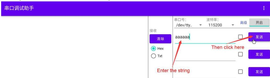
9) As shown in the figure below, if the serial port debugging assistant can receive the sent string, it means that the serial port can be used normally
