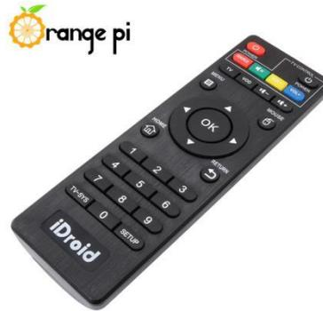
5) Then enter the **ir-keytable -t** command in the terminal, and then use the infrared remote control to press the button on the infrared receiver of the Orange Pi development board to see the received key code in the terminal
