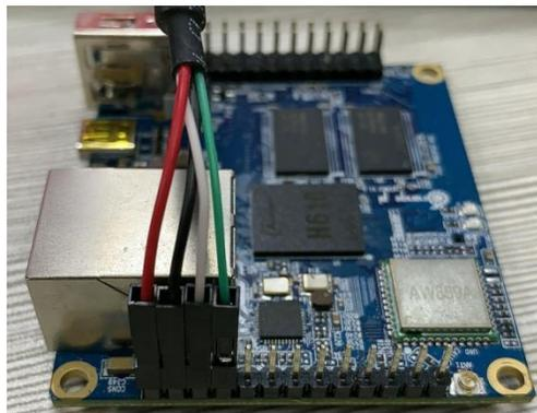
d. The wiring of USB3 is as follows
