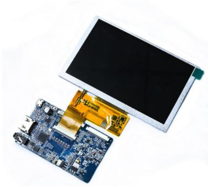
2) Then use the Micro HDMI cable to connect the Micro HDMI port of the development board to the HDMI port of the adapter board. The screen needs to be powered separately. Please insert a 5V/2A power supply into the Micro USB port of the adapter board.
