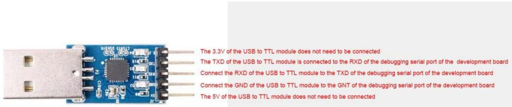
2) The corresponding relationship between the debug serial port GND, TX and RX pins of the development board is shown in the figure below
