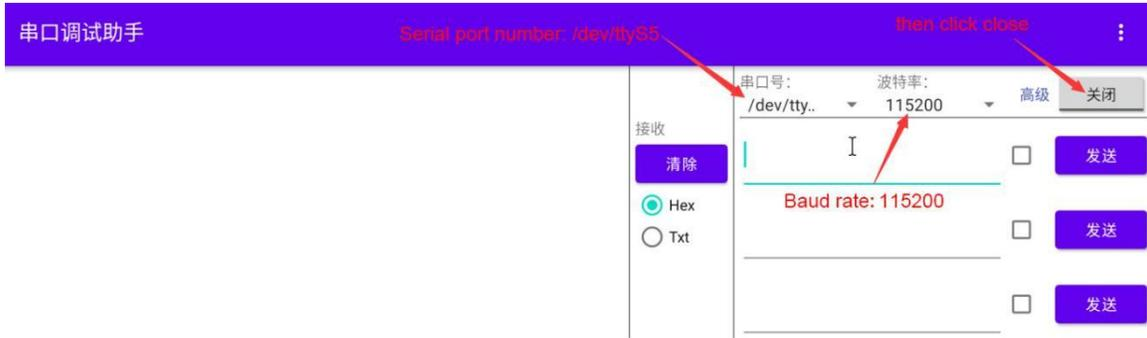
8) Then you can send a string to test the loopback function of the serial port to see if the serial port can receive the sent string
