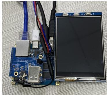
3) After connecting the LCD display to the development board, use the following command to load the `fbtft_device` kernel module
