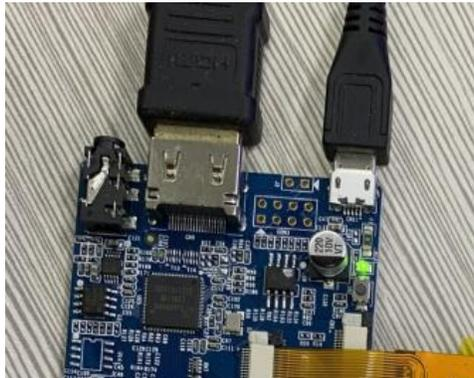
3) Modify the HDMI output resolution in **/boot/orangepiEnv.txt** to 480p, the length and width of the Framebuffer can be set to 800x480, if set to 1280x720, the font displayed on the TFT LCD screen will be very small
