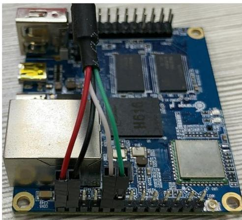
e. If you need to connect two USB devices on the 13pin interface at the same time, you will find that the 5V and GND pins on the 13pin interface are not enough. At this time, one of the USB devices can use the 5V and GND pins in the 26pin interface. The location is as shown below shown:
