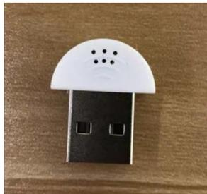
2) First insert the USB microphone into the USB interface of the development board
