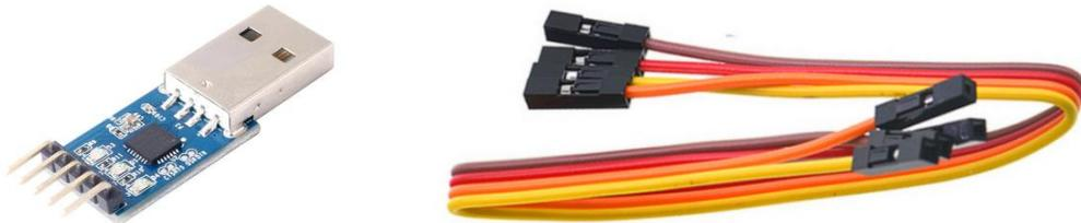
**Note that the TTL level used by the development board is 3.3v. Except for the USB to TTL module shown in the figure above, other similar 3.3v USB to TTL modules are generally available.**
