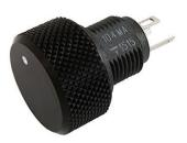
The P16S is a revolutionary concept in panel mounted potentiometers. This unique design consists of a knob driving and incorporating a cermet potentiometer. Only the mounting hardware and terminals are situated on the back side of the panel reducing to a minimum the required clearance.
