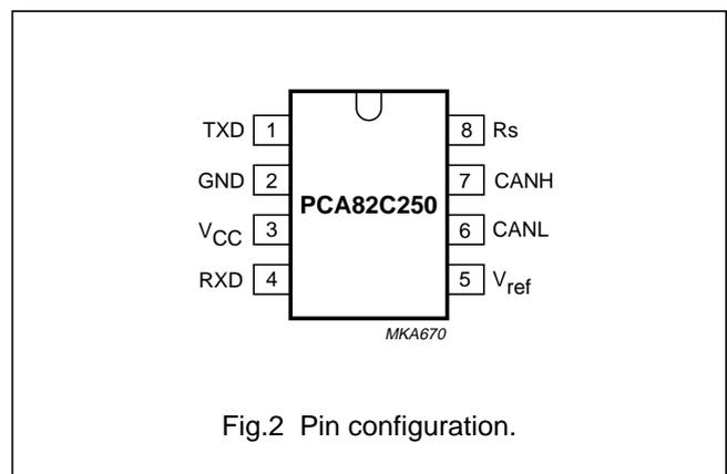
Fig.2 Pin configuration.
