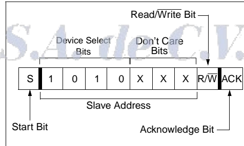
FIGURE 7-5: CONTROL BYTE FORMAT
