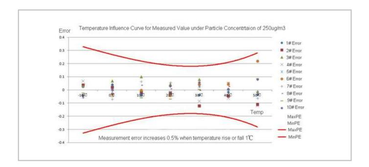
Particle measured error: under  $25\pm2^{\circ}$ C,  $0\sim1,000~\mu\text{g/m}^{3}$ , consistency and accuracy of PM1.0/PM2.5 is either  $\pm15\%$  reading or  $\pm15\mu\text{g/m}^{3}$ , the bigger one is considered.
