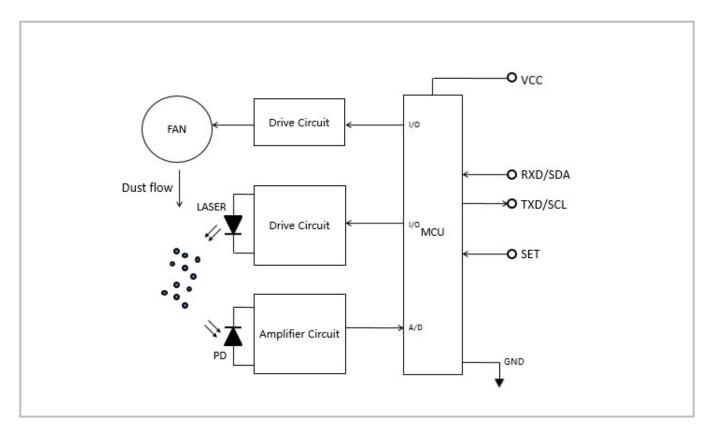
When the fan works, it will generate airflow. When the particles in the sampled gas pass through the beam of the light source (laser), a light scattering phenomenon occurs, and the scattered light is converted into an electrical signal (ie, a pulse) by the photoelectric converter. The larger the particle size, the larger the amplitude of the pulse signal output.
