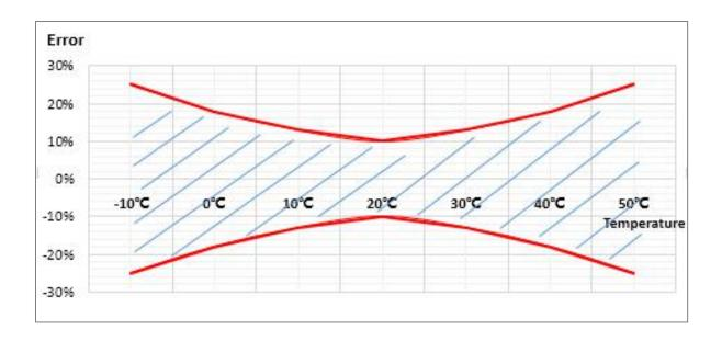
Particle measured error: under  $25\pm2^{\circ}$ C,  $50\pm10^{\circ}$ RH,  $0\sim1000\mu$ g/m<sup>3</sup>, consistency and accuracy of PM1.0/PM2.5 is  $\pm10^{\circ}$  reading or  $\pm10\mu$ g/m<sup>3</sup>, use the biggest one(TSI-8530, Cigarette)
