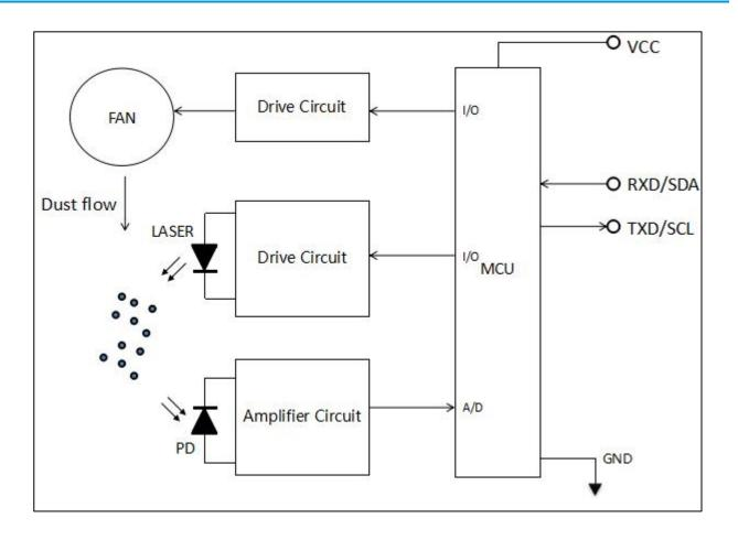
According to the above figure, The light source part of PM2012SE-A is composed of a laser tube and a driving circuit. The detection part of the sensor is composed of light sensitive part which receives reflected light and amplifying circuit. Data processing and communication output are completed by microprocessor.
