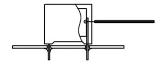
Temperature monitored inside the capacitor.
