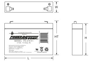
Tolerances are +/- 0.04 in. (+/- 1mm) and +/- 0.08 in. (+/- 2mm) for height dimensions. All data subject to change without notice.
