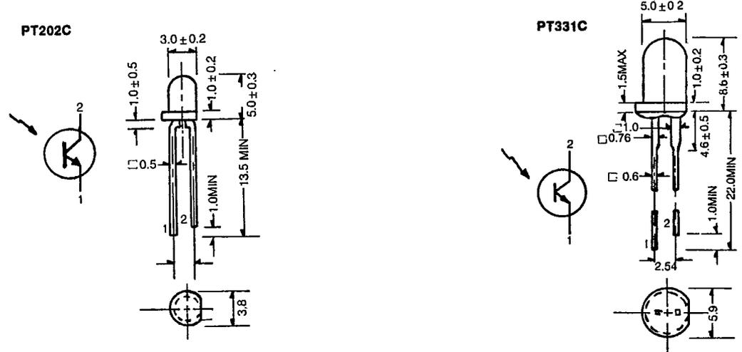
NOTE: 1 All dimensions are in millimeters. 2. Lead spacing is measured where the leads emerge from the package. 3. Protruded resin under flange 1.5 mm (0.059") Max.
