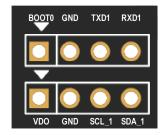
Figure 5: J21 and J18 (I2C and UART) pin header label in bottom side
