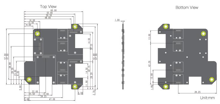
Figure 10: RAK19011 board dimensions
