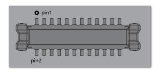
Figure 8: WisBlock 24-pin module connector
