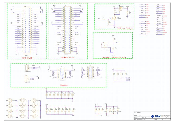
Figure 13: RAK19011 schematic diagram 1
