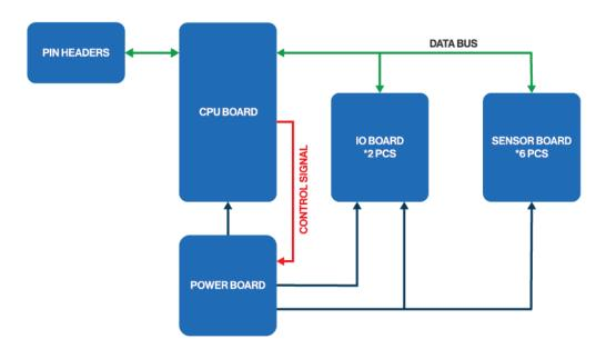
Figure 2: RAK19011 WisBlock Base block diagram
