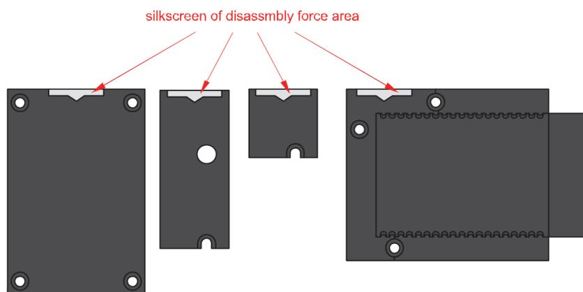
Figure 4: Detaching silkscreen on the WisBlock module
