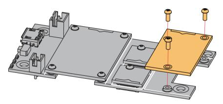
Figure 4: RAK13007 mounting connection to WisBlock Base module
