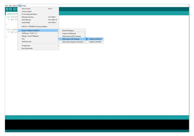
Figure 9: Selecting RAK4631 as WisBlock Core
