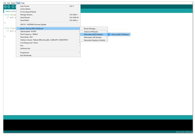
Figure 10: Selecting RAK11200 as WisBlock Core
