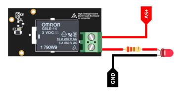
Figure 8: RAK13007 switching the LED
