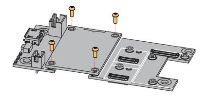
Figure 5: Removing screws from the WisBlock module
