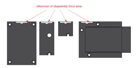
Figure 6: Detaching silkscreen on the WisBlock module
