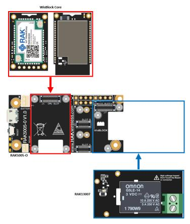
Figure 3: RAK13007 connection to WisBlock Base
