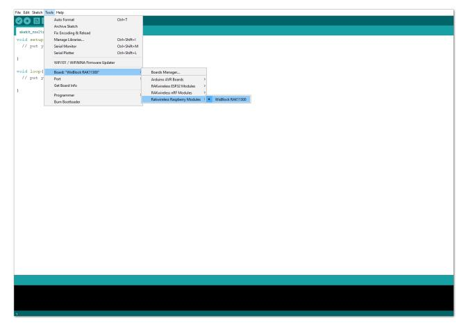
Figure 11: Selecting RAK11310 as WisBlock Core
