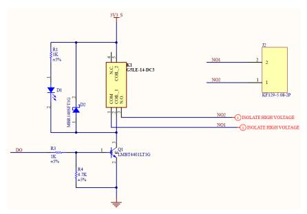
Figure 9: RAK13007 WisBlock Relay Schematic
