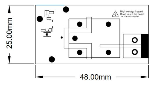
Figure 6: RAK13007 Mechanical Dimensions
