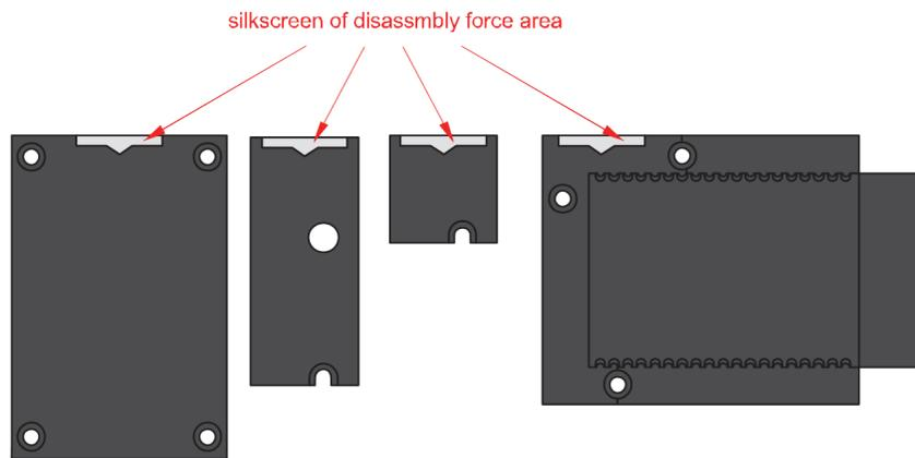
Figure 5: Detaching silkscreen on the WisBlock module
