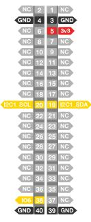
Figure 2: RAK14002 WisBlock Touch Sensor Module Pinout
