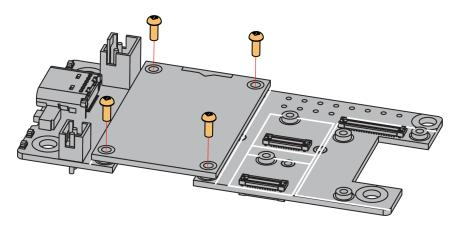
Figure 18: Removing screws from the WisBlock module
