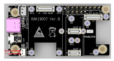
Figure 22: Solar panel connector VIN and GND
