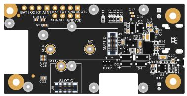
Figure 2: WisBlock Base Board 2nd Gen bottom view
