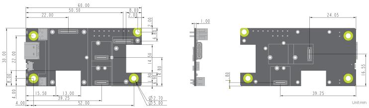
Figure 11: RAK19007 mechanical dimensions
