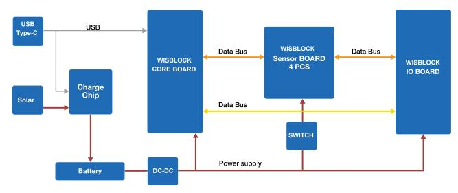
Figure 1: RAK19007 WisBlock Base Board 2nd Gen block diagram
