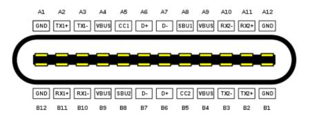
Figure 6: USB Type-C receptacle pinout
