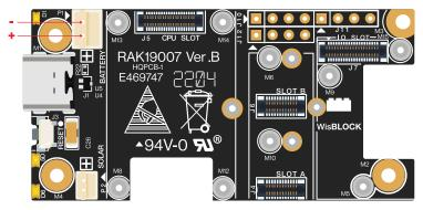
Figure 7: Battery connector pin order
