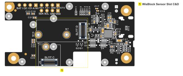
Figure 5: RAK19007 bottom view components
