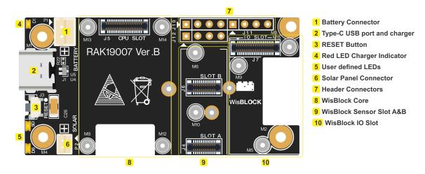
Figure 4: RAK19007 top view components
