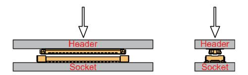
Figure 4: Alignment of WisBlock Connector
