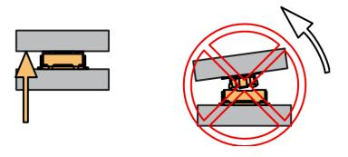
Figure 13: Wrong way: Do not rotate the header
