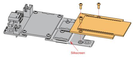
Figure 16: WisBlock IO silkscreen on the RAK19007 Base Board
