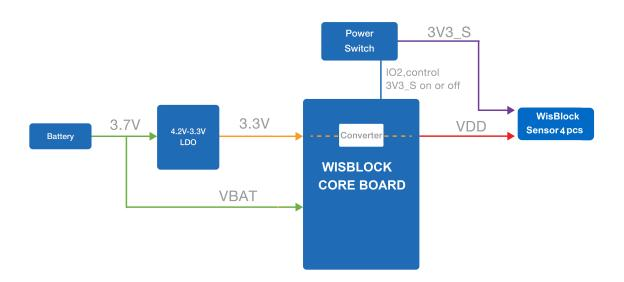
Figure 2: Power supply block diagram
