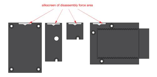
Figure 19: Detaching silkscreen on the WisBlock module
