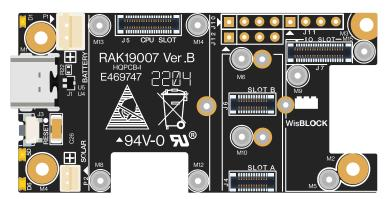
Figure 1: WisBlock Base Board 2nd Gen top view
