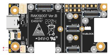
Figure 8: Solar panel connector V+ and V- Order
