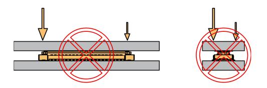
Figure 8: Avoid applying uneven forces
