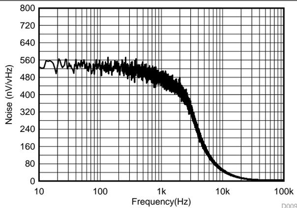
Figure 9. Noise Performance 10 Hz to 10 kHz
