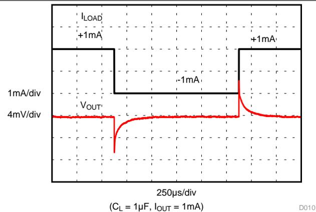
Figure 10. Load Transient
