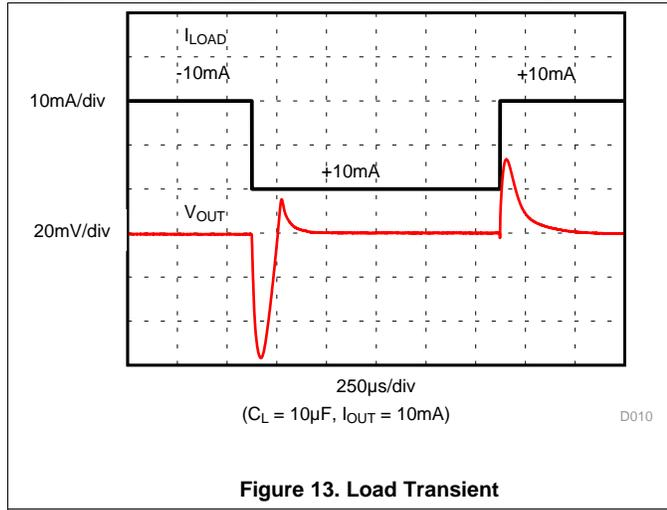
Figure 13. Load Transient
