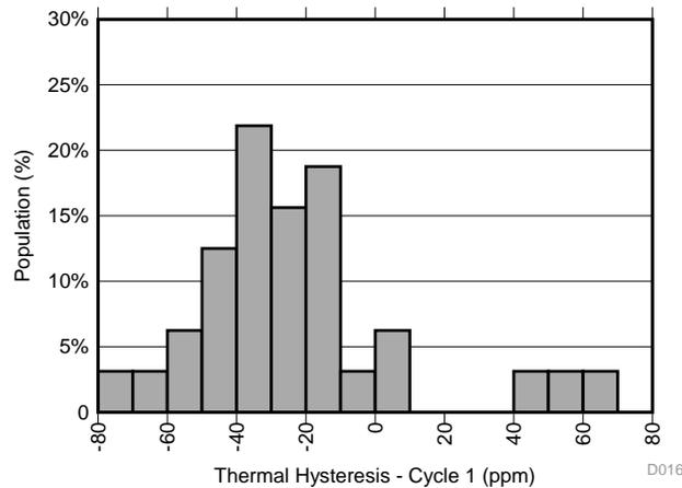
Figure 26. Thermal Hysteresis Distribution (V<sub>REF</sub>)
