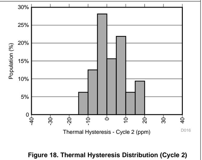
Figure 18. Thermal Hysteresis Distribution (Cycle 2)
