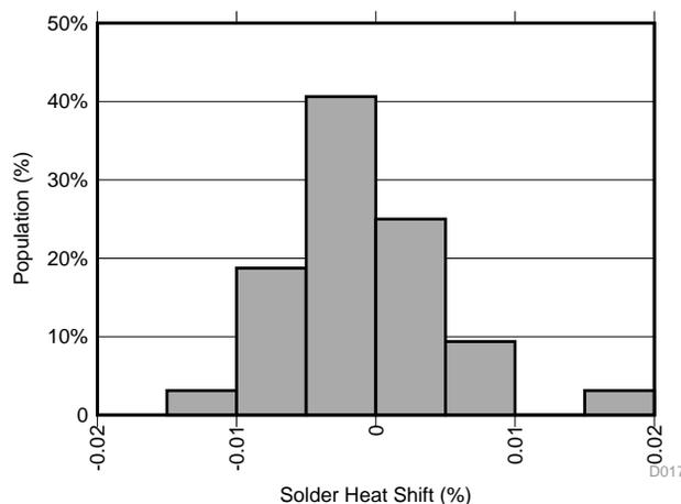
Figure 24. Solder Heat Shift Distribution,  $V_{REF}$  (%)
