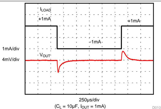
Figure 11. Load Transient
