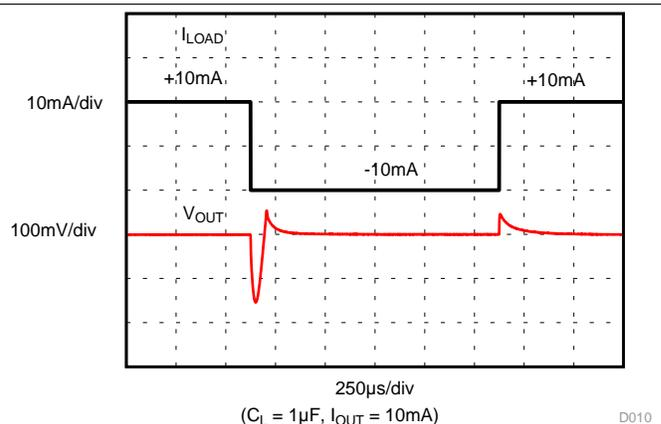
Figure 12. Load Transient
