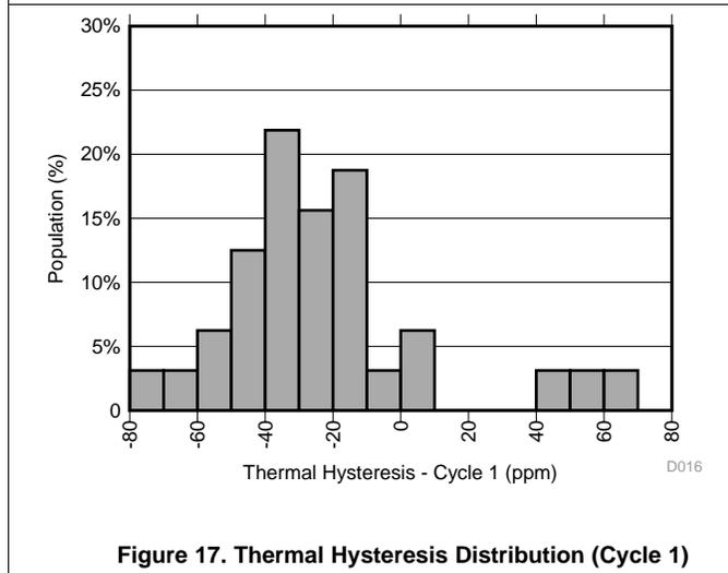
Figure 17. Thermal Hysteresis Distribution (Cycle 1)
