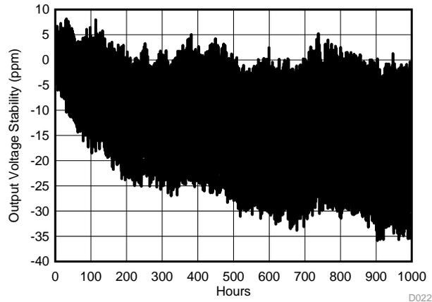
**Figure 25. Long Term Stability - 1000 hours ( $V_{REF}$ )**
