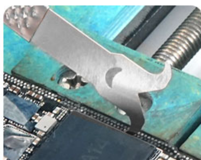
Remove IC/tap rubber
