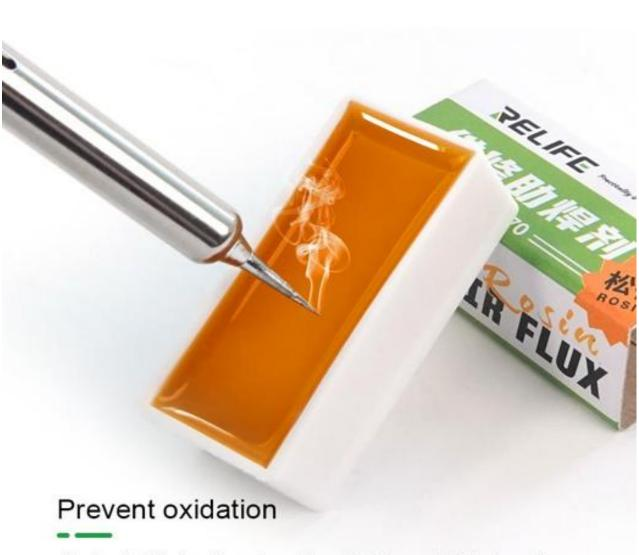
After it melts, it floats on the surface of the solder to form an isolation layer, thus preventing the oxidation of the soldering surface
